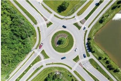
Roundabouts serve as another option to four way stops. They are circular intersections where traffic travels counterclockwise around a center island. Travelers typically travel at a speed of 15-20 mph.
